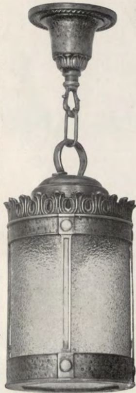
Fixture: No. 650 Length: 19 inches Diameter of Lantern: 5½ inches Finish: Swedish Iron Antique Hammered Bronze Weathered Brass Light amber rippled glass panels and bottom May be used with 40 to 100 watt Mazda lamps
